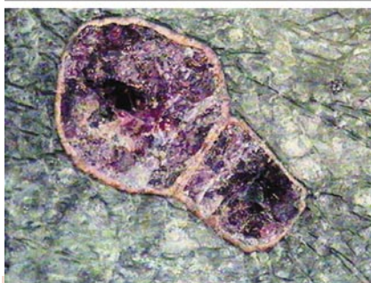
Remnants of a garnet harzburgite diamond parent rock (light green) are disseminated through this kimberlite (dark blue). Pyrope is the largest fragment in detail a light brown kelyphite rim.
