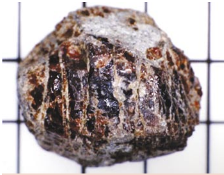
A pyrope nearly 3 cm in diameter has numerous parting planes that are altered. This grain will break down quickly in the secondary environment to produce indicator grains only a few millimetres in diameter.
